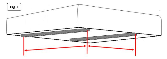
**Step-2** Using the noted measurements of the aluminum track system rails on the underside of your tent, determine the placement of the Quick Release Tent Bracket assembly on your SRM Rack crossbars or Overland Rack crossbars.
