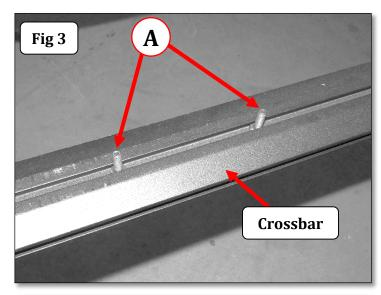
**Step-4** Align the (2) ¼" x ¾" hex bolts installed in the crossbar with the (2) holes in the base bracket of the Quick Release Tent Bracket assembly, and position the base bracket on the crossbar so the ¼" x ¾" hex bolts are protruding through the holes in the base bracket, (Fig 4).
