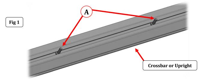
**Step-3** Align the  $\frac{1}{4}$ " x  $\frac{3}{4}$ " hex bolts installed in the crossbars or uprights with the holes in the Overland Series Gear Accessory Plate, and position the Overland Series Gear Accessory Plate on the crossbars or uprights so the  $\frac{1}{4}$ " x  $\frac{3}{4}$ " hex bolts are protruding through the attachment holes in the Overland Series Gear Accessory Plate.
