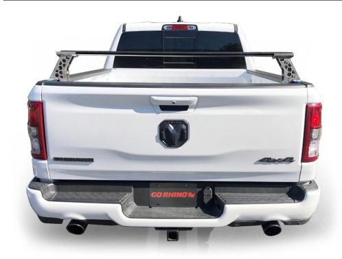
Once you position each tower and cross bar to your desired location, fasten all loose hardware. If bowing is present on the crossbars, loosen all hardware from the towers to the rail and make sure the cross bar is flat on the tower. Over tightening the tower onto the bed rail can result in cross bar bowing. Periodically inspect hardware and fasten as needed.
