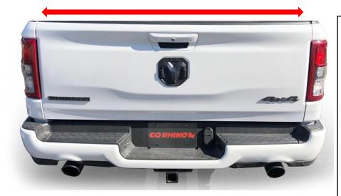
Measure the inside bed rail distance. Use that distance to determine the spacing for the XRS towers.
