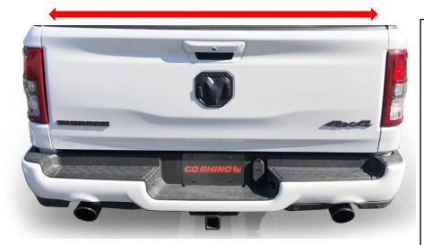
Measure the inside bed rail distance. Use that distance to determine the spacing for the SRM towers.
