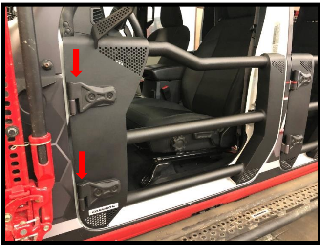
Loosen hinge fasteners
