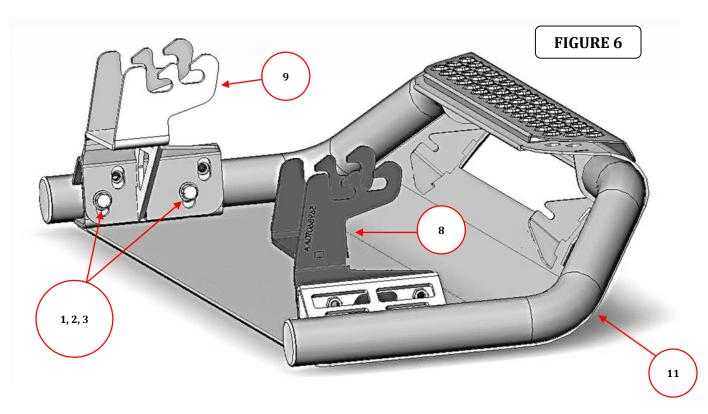
**Step-8** With assistance align and hold the RC3 or RC4 front guard in the desired position on the vehicle, then tighten all OEM and supplied nuts and bolts.
