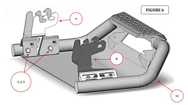
**Step-8** With assistance align and hold the RC3 or RC4 front guard in the desired position on the vehicle, then tighten all OEM and supplied nuts and bolts.
