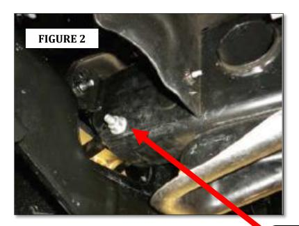
Remove nut and bolts securing the driver side tow hook to the frame.
