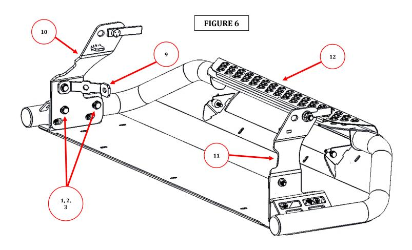
**Step-8** With assistance align and hold the RC3 front guard in the desired position on the vehicle, then tighten all OEM and supplied nuts and bolts.
