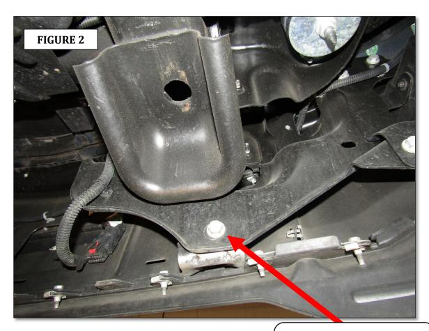
Remove bolt securing the OEM bumper to the inner bumper bracket.
