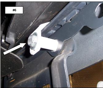
Repeat the above steps to install the passenger side lower and upper brackets.
