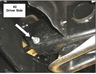
**Step-2** Shift the front tow hook bolt toward the center of the vehicle, then from the tow hook opening, slide the vehicle attachment end of the driver side main bracket under the frame, and rotate the bracket, (**Photo 3 & 4**).
