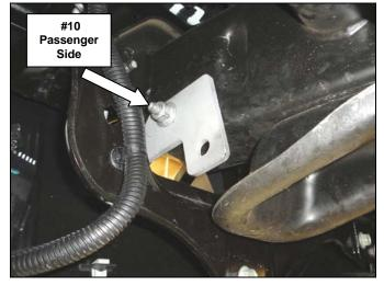
**Step-6** Attach the passenger side auxiliary bracket to the side of the frame using the tow hook rear bolt and to the passenger side main bracket using (1)  $\frac{1}{2}$ " x 1  $\frac{1}{2}$ " hex bolt, (1)  $\frac{1}{2}$ " flat washer, (1)  $\frac{1}{2}$ " lock washer and (1)  $\frac{1}{2}$ " hex nut, (**Photo 11 & 12**). Leave the factory and supplied nuts and bolts loose for final adjustment.
