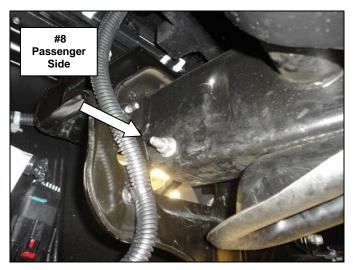
**Step-5** From the tow hook opening, slide the vehicle attachment end of the passenger side bracket under the frame, rotate the bracket and position the upper attachment hole in the bracket over the shank of the front tow hook bolt and reinstall the nut, (**Photo 9 & 10**). Leave the nut and bolt loose for final adjustment.
