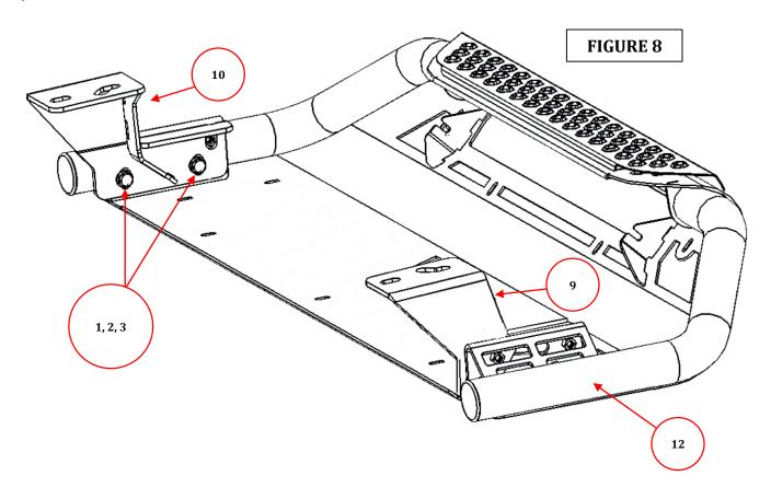
**Step-10** With assistance align and hold the RC3 or RC4 front guard in the desired position on the vehicle, then tighten all OEM and supplied nuts and bolts.
