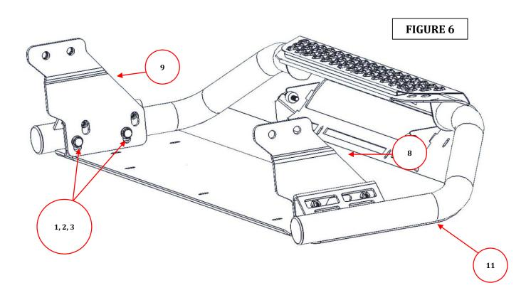
**Step-7** With assistance align and hold the RC3 front guard in the desired position on the vehicle, then tighten all OEM and supplied nuts and bolts.
