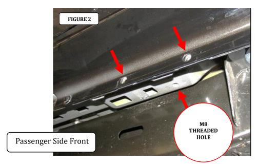
**Step-2** Attach one front brackets to the pinch mold using (2) 1/4" x 1" hex head bolts, (4) 1/4" flat washers, (2) 1/4" lock washers and (2) 1/4" hex nuts, and to the underside of the body using (1) M8 x 25mm hex bolt, (1) 5/16" lock washer and (1) 5/16" flat washer, (FIGURE 3 & 4). Leave the nuts and bolts loose for final adjustment.
