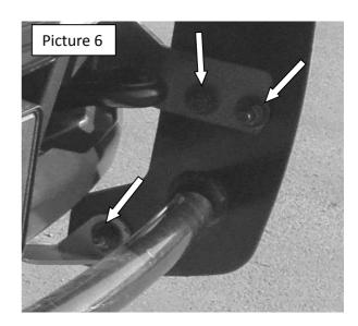
**Step-6** Attach the side plates to the lower brackets using (1) 1/2" X 1 1/2" hex bolts, (1)  $\frac{1}{2}$ " flat and lock washers and (1)  $\frac{1}{2}$ " hex nut by each side. Do not tighten. Picture 6.
