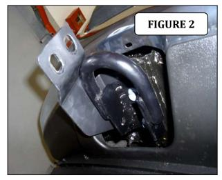
**Step-3** Slide the main bracket between the rear's tow hook bolt and frame then re-install the tow hook over the main bracket. Re-attach using the factory bolts removed in previous step. Figure 2. Leave loose. Follow to step 8.
