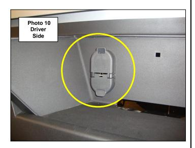
**Step-11** Reconnect the factory bumper wiring harness to the sensors and to the vehicle wiring harness.
