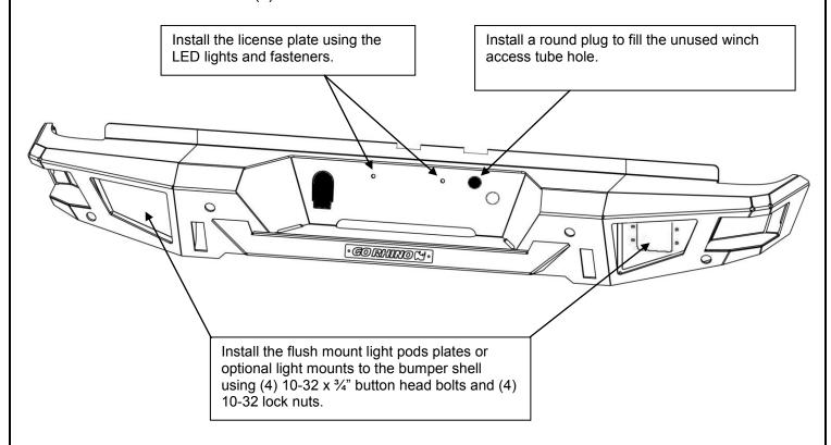
Step-15 Remember to check and retighten all factory and supplied nuts and bolts periodically.
