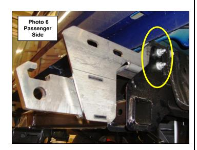
**Step-8** With assistance attach the bumper shell brackets to each frame bracket using (2) ½" x 1 ½" hex bolts, (4) ½" flat washers, (2) ½" lock washers and (2) ½" Hex nuts, Align the bumper shell with the vehicle, verify that the tailgate clears when lowered, and tighten all nuts and bolts, (Photo 7 & 8).
