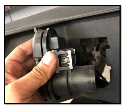
Reinstall OEM trailer plug. Refer to OEM manual on how to remove from the OEM bumper.
