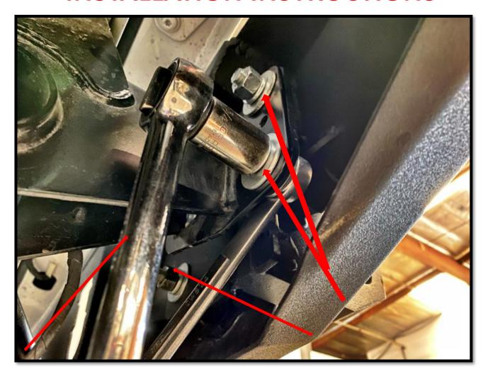
Begin to fasten ½" hardware with ¾" wrench or socket. Be sure to fasten all four nuts (4 per side). Begin to align bumper to square up with the bed.
