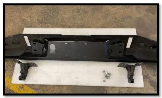
Lay bumper on a protective surface to prevent finish from damage. You'll need to preassemble the rear brackets onto the bumper. Determine where each bracket goes on the backside of the bumper.
