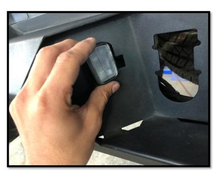
Reinstall OEM license plate lights (left and right). Refer to OEM manual on how to remove from the OEM bumper.
