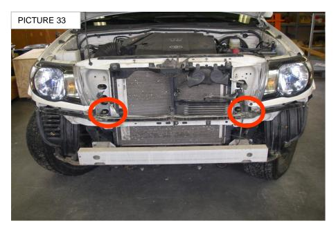
**Step-19** Remove 2 k lath screws on lower back of front grill, put the bracket grill and install the k lath screws from hardware kit (**don't tight**), re install the front gril, re install the 4 (10mm)nut. (PICTURE 34)
