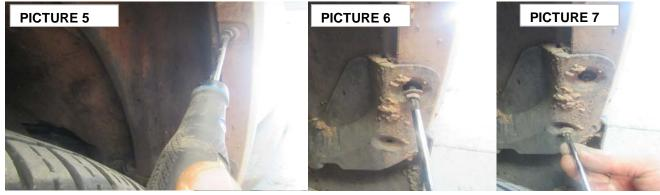
Step-5 Remove the down lower cover screw & all bottom deflector screws. (PICTURE 8)
