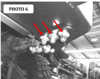
**Step-5** Adjust the mounting plate/winch tray and brackets to the forward position, center and level the mounting plate/winch tray with the vehicle frame then tighten all factory hex nuts securing the frame brackets, and the supplied nuts and bolts securing the mounting plate/winch tray and frame brackets. Do not tighten the auxiliary and extension bracket nuts and bolts at this time.
