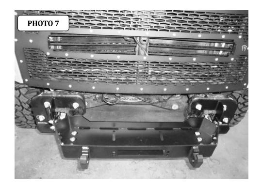
**Step-6** If you are installing a winch, place the winch in the mounting plate/winch tray and refer to the winch manufacturer's instructions for installation. Do not install the fairlead at this time.
