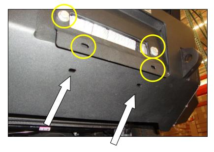
If installing a winch, attach the license plate directly to the (2) obround holes in the lower face of the bumper shell using the supplied ¼" bolts and nuts. Remember to check and retighten all factory and supplied nuts and bolts periodically.
