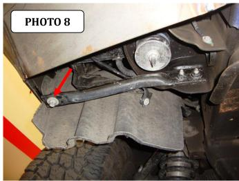
**Step-15** With assistance, adjust and hold the bumper shell visual alignment position, then tighten all factory and supplied nuts and bolts. Note: It may be necessary to loosen the nuts and bolts securing the mounting plate/winch tray and brackets.
