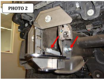
**Step-11** Position the mounting plate/winch tray on top of the auxiliary brackets. Align the holes and secure the mounting plate/winch tray to each frame bracket using (2) ½" x 1 ½" carriage bolts, (2) ½" flat washers, (2) ½" lock washers and (2) ½" hex nuts, and to each auxiliary bracket using (3) ½" x 1 ½" carriage bolts, (3) ½" flat washers, (3) ½" lock washers and (3) ½" hex nut, (Photo 3 & 4).
