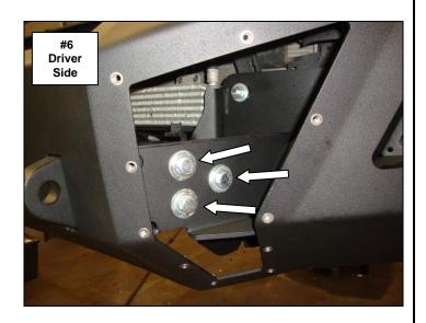
**Step-6** Align the holes and attach each bumper support bracket to the vehicle frame using (2) 3/8" x 1  $\frac{1}{4}$ " hex bolts, (2) 3/8" flat washers, (2) 3/8" lock washers and (2) 3/8" hex nuts, and to the replacement bumper bracket using (1)  $\frac{1}{2}$ " x 1  $\frac{1}{2}$ " hex bolt, (2)  $\frac{1}{2}$ " flat washers, (1)  $\frac{1}{2}$ " lock washer and (1)  $\frac{1}{2}$ " hex nut, (Photo 7).
