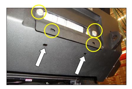
Remember to check and retighten all factory and supplied nuts and bolts periodically.
