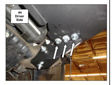
**Step-4** Center the mounting plate/winch tray with the vehicle then tighten the nuts and bolts securing the auxiliary brackets to the frame. Finger tighten all factory and supplied nuts and bolts securing the mounting plate/winch tray and frame brackets.
