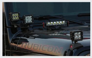
Light mounts allow for installation of lights to the hood hinge, lower A-pillar, the upper cowl, hood clamp, or hard top.
