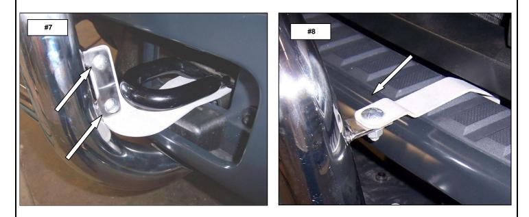
**Step-8** Align the Rhino Charge bar and bracket assembly and tighten all nuts and bolts. Remember to check and re-tighten the hardware periodically.
