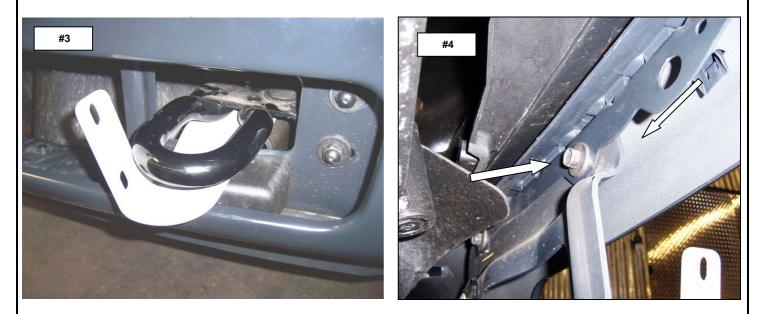
**Step-4** Position one of the upper brackets behind the bumper, so the longer leg of the bracket extends out between the top of the bumper and the bottom of the grille. **Photo #5**
