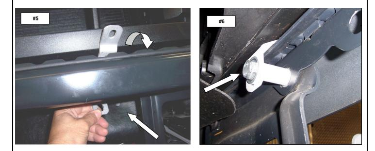
Repeat the above steps to install the passenger side lower and upper brackets.
