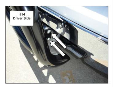
**Step-8** Align the RC2 Bull Bar with the vehicle and tighten all factory and supplied nuts and bolts. Remember to check and retighten the nuts and bolts periodically.
