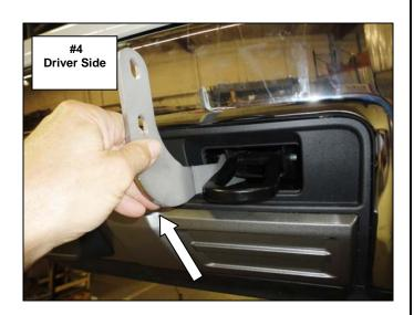
**Step-3** Hook the slot in the bracket over the shank of the front tow hook bolt, reinstall the front bolt nut and rear tow hook bolt to secure the bracket to the side of the frame, (**Photo 5**). Leave the nut and bolts loose for final adjustment.
