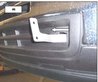
Step-3 Align the bracket with the tow hook holes in the frame and install (1) ½" rod bolt into the frame, so the threads extend out through the rear tow hook mounting hole and bracket. **Photo #7 & #8**
