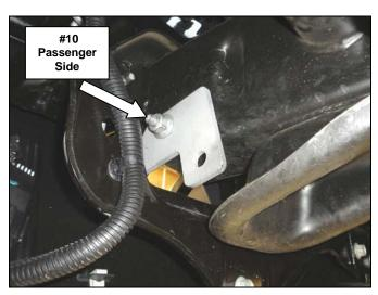
**Step-6** Attach the passenger side auxiliary bracket to the side of the frame using the tow hook rear bolt and to the passenger side main bracket using (1) ½" x 1 ½" hex bolt, (1) ½" flat washer, (1) ½" lock washer and (1) ½" hex nut, (**Photo 11 & 12**). Leave the factory and supplied nuts and bolts loose for final adjustment.
