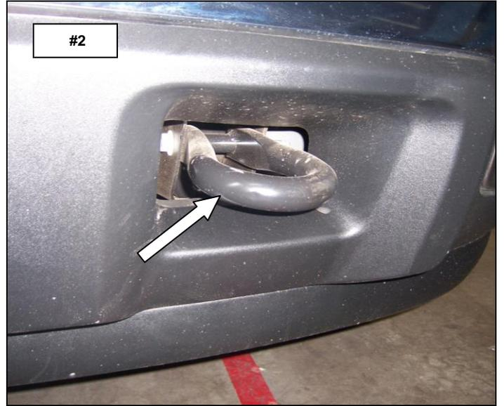
**Step-2** From behind the bumper valance, position the driver side bracket so the leg of the bracket extends out through the tow hook opening, then rotate and align the bracket with the side and bottom of of the frame. **Photo #3 & #4**
