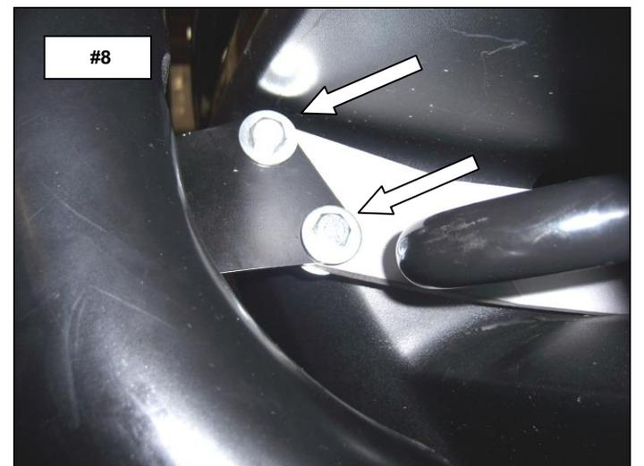
**Step-5** Align the Charger Bull Bar and bracket assembly, and tighten all nuts and bolts.
