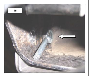
**Step-4** Install (1)  $\frac{1}{2}$ " x 5  $\frac{1}{2}$ " hex bolt with (1) flat washer through the bracket and front tow hook mounting holes. Secure the bracket using (2)  $\frac{1}{2}$ " flat washers  $\frac{1}{2}$ " (2) lock washers and (2)  $\frac{1}{2}$ " hex nuts.Leave the nuts and bolts loose for final adjustment. **Photo #9 & #10**
