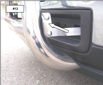
**Step-6** Align the Rhino Charger bar, bracket assembly and tighten all nuts and bolts. Remember to check and re-tighten the hardware periodically.
