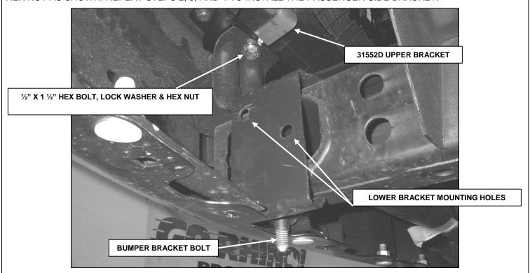
**STEP-5** LOCATE THE HOLES IN THE BUMPER BRACKET. THESE HOLES WILL SERVE AS THE LOWER BRACKET MOUNTING POINTS.
