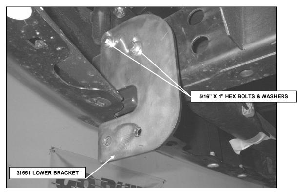
**STEP-7** LOOSELY ATTACH ONE OF THE 31551 LOWER BRACKETS TO THE BUMPER BRACKET USING 5/16" X 1" HEX BOLTS, FLAT WASHERS AND LOCK WASHERS. REPEAT STEPS 5, 6, AND 7 TO INSTALL THE PASSENGER SIDE.
