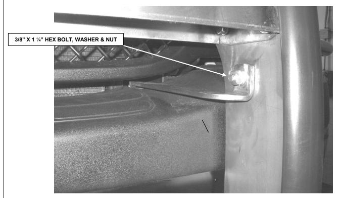
**STEP-8** ATTACH THE GRILLE GUARD ASSEMBLY TO THE UPPER BRACKETS USING THE 3/8 X 1" HEX BOLTS, LOCK WASHERS, FLAT WASHERS AND HEX NUTS.
