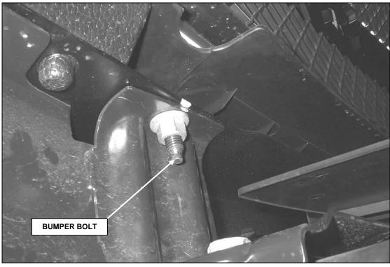
**STEP-2** BEGINNING WITH THE DRIVER SIDE, REMOVE THE NUT AND UPPER BUMPER BOLT. THE BOLT IS LOCATED ON THE BACK EDGE AT THE TOP OF THE BUMPER. THIS LOCATION WILL SERVE AS THE UPPER BRACKET MOUNTING POINT.
