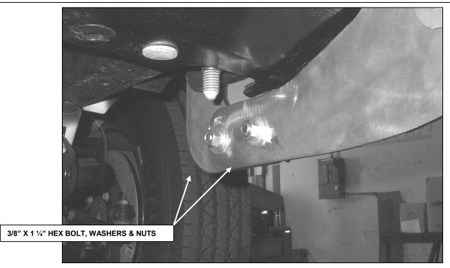
STEP-8 ATTACH THE GRILLE GUARD ASSEMBLY TO THE LOWER BRACKETS, USING THE 3/8" x 1 1/4" HEX BOLTS, LOCK WASHERS, FLAT WASHERS AND HEX NUTS.
