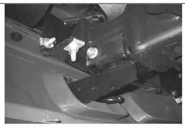
STEP 4. POSITION 1024CP FRAME BRACKET OVER THE SHANK OF THE UPPER BOLT, AND ATTACH IT TO THE BOTTOM AND SIDE OF THE FRAME USING THE FACTORY LOWER BOLT AND NUT.
