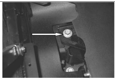
**STEP 1.** BEGINNING WITH THE PASSENGER SIDE, LOCATE AND REMOVE THE UPPER BUMPER BOLT. THE BOLT IS LOCATED BEHIND THE GRILLE ON THE TOP OF THE BUMPER. THE BOLT IS ACCESSIBLE BY REMOVING THE RIVETS AND PLASTIC TRIM PANEL ON TOP OF THE GRILLE, AND REACHING DOWN THROUGH THE OPENING.
