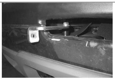
STEP 2. POSITION 1100AP UPPER BRACKET THROUGH THE OPENING IN THE BUMPER. LOOSELY ATTACH THE BRACKET TO THE BUMPER USING THE 12MM X 70MM BOLT, TUBULAR SPACER AND  $\frac{1}{2}$ " WASHERS.
