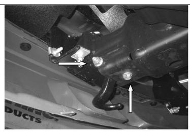
STEP 3. LOCATE THE PASSENGER SIDE TOW HOOK MOUNTING BOLTS. REMOVE THE BOLT FROM THE BOTTOM AND THE HEX NUT FROM THE UPPER BOLT THAT PASSES THROUGH THE SIDES OF THE FRAME.
