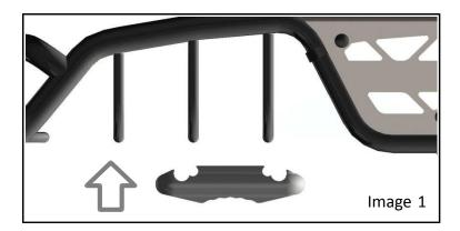
3. Place the Safari Rack with the plastic holders above the roof bars of your vehicle\*. Note 1: It may be necessary to slide and relocate the roof bars to allow the installation.
