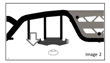
4. Place the (x4) fixation plates above the cross tubes, align them with each plastic holder, then place the (x4) "U"-bolts below the roof bars.
