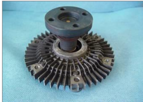
Fan clutch bearing blocked → breakage
