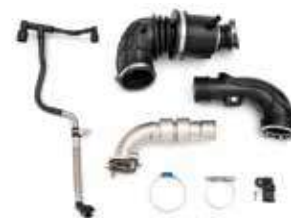
19332838 LTG Rear Wheel Drive Engine Completion Kit • Includes required PCV hose • Includes duct assembly for turbo inlet, throttle body inlet and turbo outlet tubes • Includes all clamps and inlet air pressure sensor • Does not include charge air cooler
