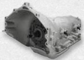
19300175 SuperMatic™ 4L85-E Four-Speed Automatic Transmission Features five-pinion gearsets, heat-treated stator shaft splines, induction-hardened turbine shaft, seven-plate clutch and specific valve-body calibration. See page 366 for torque converter applications.
