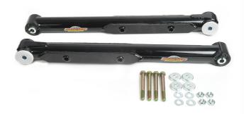
2. Your new lower control arms have a spherical bearing installed in one end of the arm. This end attaches to the frame; each bearing will have two steel spacers located one on each side of the bearing. They are already installed. Note: The recess in the control arm goes to the inside of the car. Simply slip the arm with the spacers up into the frame. Make sure the grease fitting on the rear end side of the arm is facing down towards the ground. Slide the stock bolt
