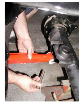
4. Once the control arms are installed, the sway bar can be positioned correctly. First slide the sway bar up into position without using the 4 spacers provided in your kit. If the bar slides up without excessive space bolt the sway bar directly to the subframe using the hardware supplied in the kit.
