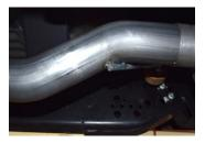
**2.** Install head pipe #A onto your existing stock front pipe and attach with clamp #G. Insert welded hanger into rubber grommet.
