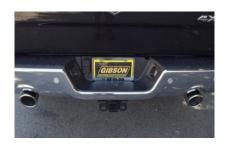
Now go back and tighten all clamps, nuts and bolts. Use stainless steel cleaner weekly to prevent tip from discoloration. Inspect all fasteners after 25-50 miles of operation and re-tighten as necessary.
