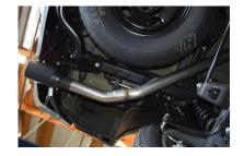
Install the Gibson Tips onto your exit pipes. Place the tips to your desired position. Be for tightening down the system it is recommended to secure the tips the position you want and check the location after each connection is tightened.
