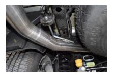
Install the driver side tailpipe # D into the muffler at least 1-1/2" to 2". This pipe will route over the axle and between the Frame rail and tire. Use clamp # H to secure pipe to the muffler. Do not tighten. Insert hangers into rubber grommet.
