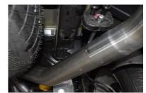
Install the passenger side tailpipe # C into the muffler at least 1-1/2'' to 2". Use clamp # H to secure pipe to muffler. Do not tighten. The tailpipes both will lean towards the driver side for clearance.
