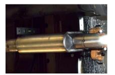
**3.** INSTALL MUFFLER # B. ONTO HEADPIPE 1½" TO 2". USE CLAMP #E TO SECURE MUFFLER TO HEADPIPE. DO NOT TIGHTEN
