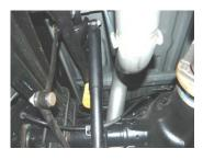
5. Install the over axle tailpipe #B onto headpipe 1.5"-2". Use clamp #D to secure. Do not Tighten
