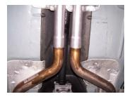
2. To remove the stock exhaust, first you must remove the factory cross member under the X pipe. Then unbolt and remove driver side tailpipe at the flange. Now unbolt and cut tack welds on factory clamps at the X pipe and carefully remove factory exhaust, save clamps for new exhaust installation. The 2.75" clamps are included in case you can't use the factory clamps. Leave all rubber grommets on hangers. Use WD-40 to help remove hangers.
