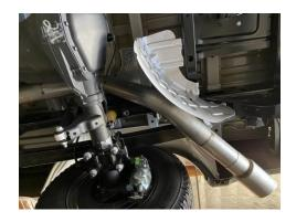
**5**. Finally, over axle pipe #C can be installed using the Band Clamp #E. Once the over axle pipe is in you may install the Tip to your desired wants. (Tighten all clamps working from front to back.)
