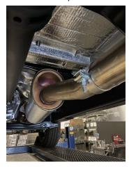
2. TO REMOVE YOUR STOCK EXHAUST, REMOVE IT FROM THE CLAMP LOCATED JUST THE RESONATOR. REMOVE HANGERS FROM RUBBER GROMMETS, USE WD-40 TO AID IN REMOVAL, LEAVE GROMMETS IN PLACE.
