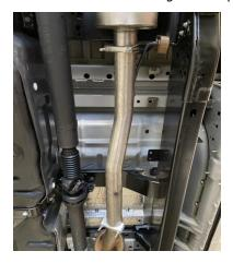
3. INSTALL HEADPIPE #A ONTO STOCK PIPE BEHIND RESONATOR. INSERT WELDED HANGER INTO RUBBER GROMMET. USE CLAMP #D PROVIDED TO SECURE. DO NOT TIGHTEN.
