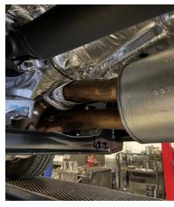
2. TO REMOVE YOUR STOCK EXHAUST, REMOVE IT FROM THE CLAMP LOCATED JUST THE RESONATOR. REMOVE HANGERS FROM RUBBER GROMMETS, USE WD-40 TO AID IN REMOVAL, LEAVE GROMMETS IN PLACE.
