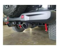
7. Adjust the tips to your preference. Make sure everything is clear of frame rails and parts and re tighten the system starting from the front clamp. Check everything after each clamp is tightened.
