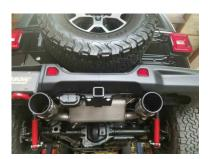
6. Slide the 2.5" band clamp over the expanded part of the muffler and make clamp snug but not tight. Install the Gibson provided tips. Check for exhaust clearance before tightening.
