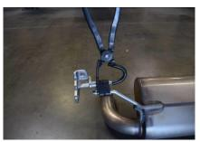
4. Remove hangers from OEM exhaust using removal pliers or large channel pliers and re-install them on the Gibson as shown. Using a lubricant can aid in the removal.
