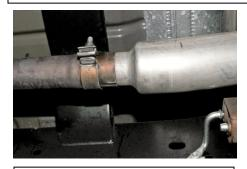
2. Install Headpipe #F onto the factory flange. You will re use the factory nuts at this connection. Loosely tighten down the flange.
