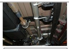
3. With the head pipe and hangers in position install the muffler assembly Item # B. You will use the Clamp Item # E to secure to the head pipe. Do not tighten keep loose.
