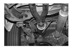
3. Install muffler assembly Item # D onto the Gibson head pipes. Slide the rubber grommet onto the welded hanger.
