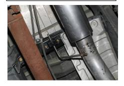
5. Install The muffler assembly Item # C Onto the resonator. Also slide the muffler hanger into the factory rubber grommet. Install the over axle pipe Item # D into the muffler outlet and install the hanger into the rubber grommets. Use clamp Item # F to secure. Do not tighten
