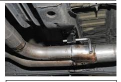
4. Install the Resonator Item #B onto the head pipe Item # A. The inlet of the resonator will have the louvers opening towards the front of the vehicle. Loosely tighten down.
