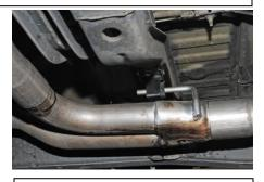
4. Install the Resonator Item #B onto the head pipe Item # A. The inlet of the resonator will have the louvers opening towards the front of the vehicle. Install extension pipe Item # J onto the resonator.
